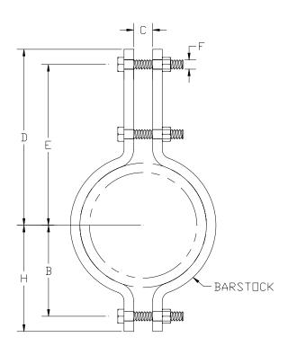
MATERIAL TYPES: Carbon Steel, chrome molybdenum or stainless steel.
